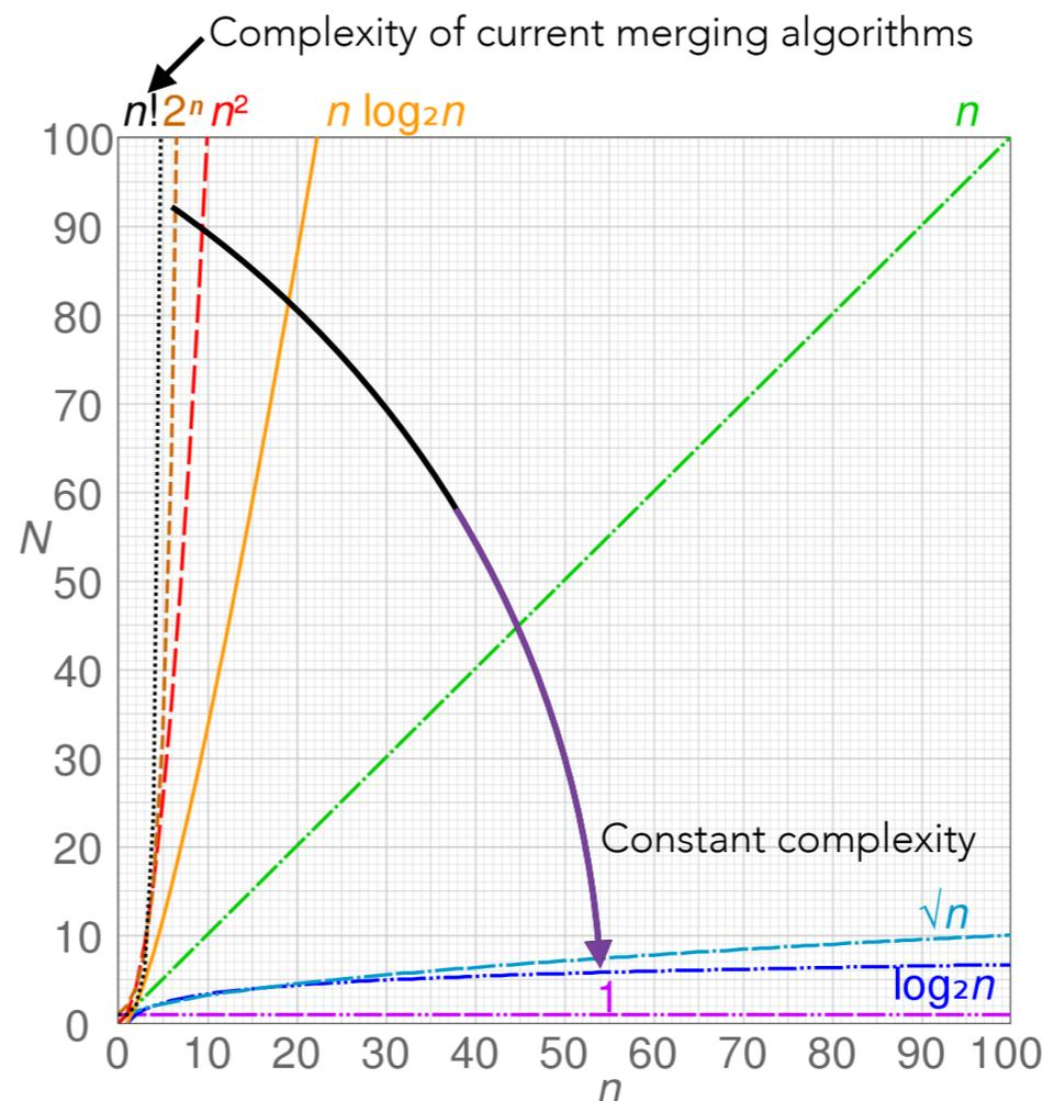
Figure 1: Number of operations,  $N$  vs number of input items,  $n$  for algorithms of common complexities, assuming a constant of 1. Polynomial ( $n^2$ ) or better scaling is usually considered efficient for complex problems, while exponential ( $2^n$ ) or factorial ( $n!$ ) scaling are infamous for being highly resource demanding. Plot from Ref. [2].
